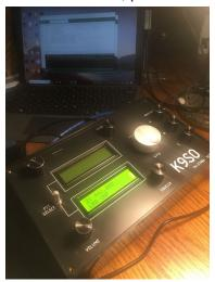
I am calling this the Ham Radio 'BusyBox' as it simply involves 8 shaft encoders and two displays that could be programmed in any way to control almost any radio with RS-232 or CI-V control features. This could even be a remote rotor controller and antenna switch control with features allowing for many other interfaces left over.
